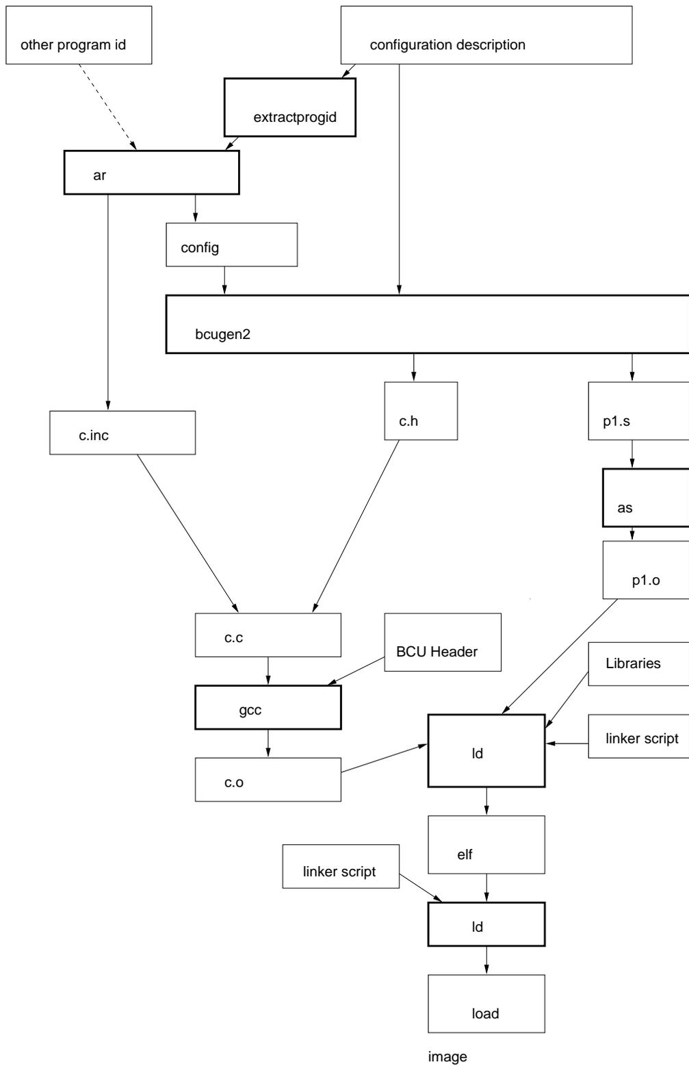
Figure 6.2.: *build.img* operational sequence and data flow
