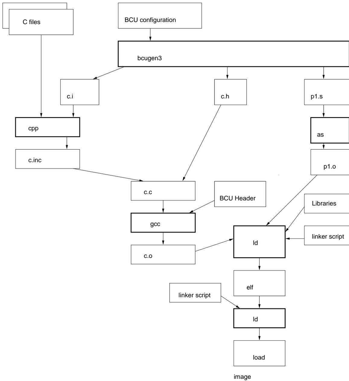
Figure 6.3.: *build.dev* operational sequence and data flow
