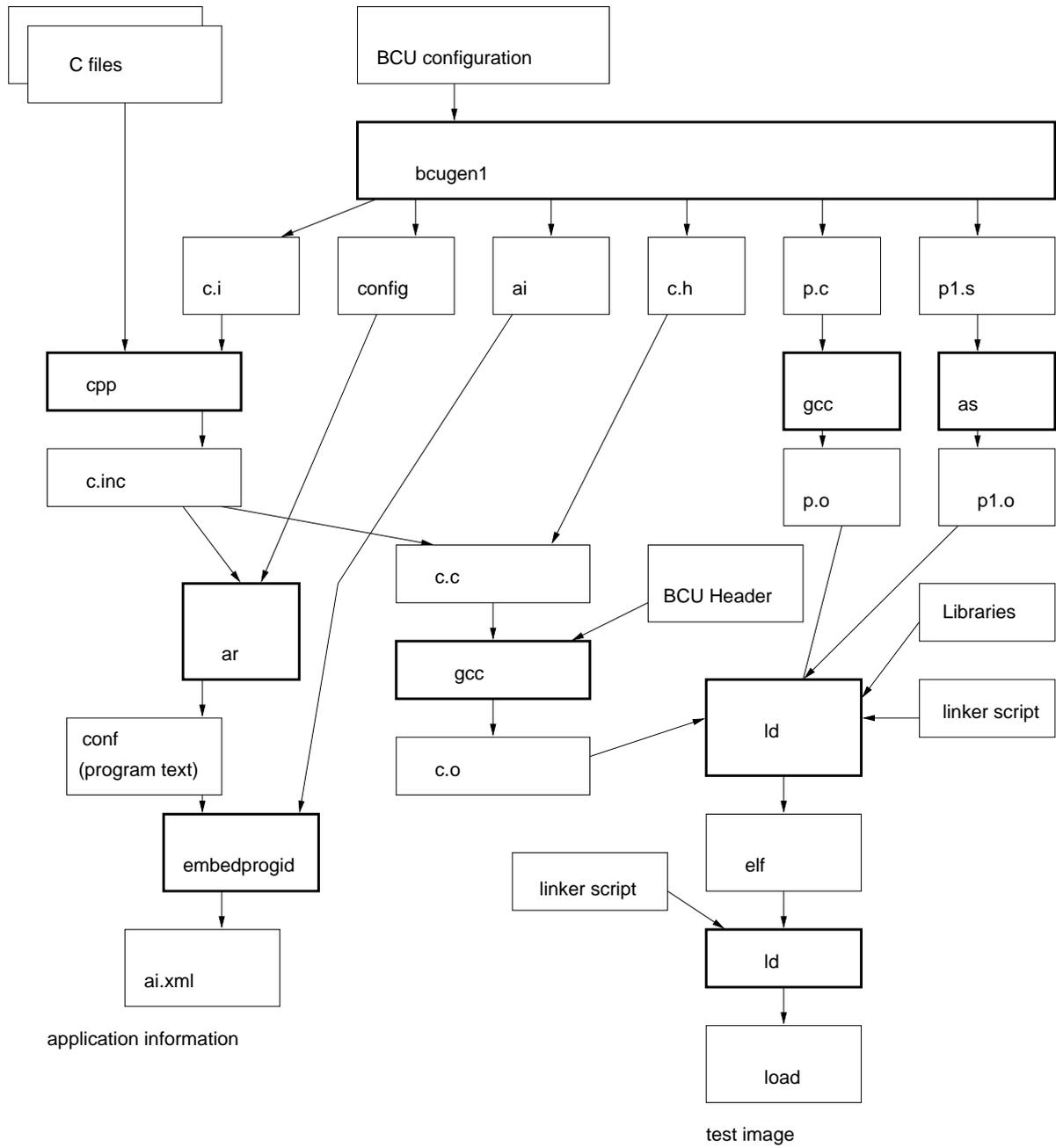
Figure 6.1.: *build.ai* operational sequence and data flow
