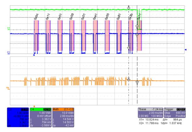
Figure 4: U\_AckInformation transmission completed in time
