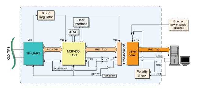
Figure 1: TP-UART interface board connected to KNX TP1 and a PC
