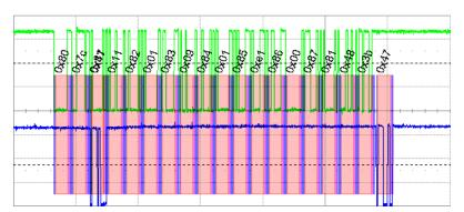
Figure 7: Corrupted control byte producing error indications
