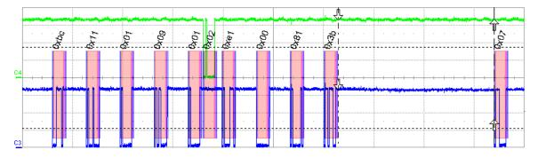
Figure 3: U\_State.request during frame reception (2.00 ms/div, 6.22 ms between cursors)
