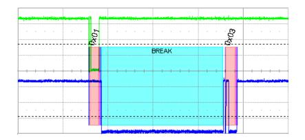
Figure 9: TP-UART software reset (2.00 ms/div)
