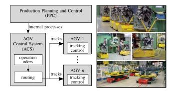
Fig. 1. This figure shows, to the left, the modules involved in a classical system. The PPC analyses general processes (e.g., costumer requests) for the ACS. The ACS identifies operation orders in internal processes and computes routing tables composed of sequences of line, arc and spline segments as tracks. A single AGV has to simply follow the tracks with a tracking control. No path planning is involved. To the right, AGVs in action on an automotive assembly line.
