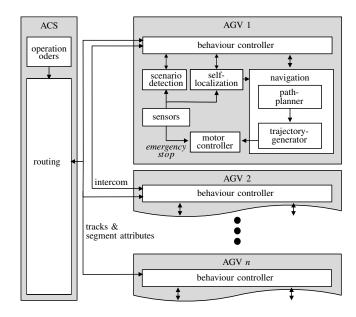
Fig. 3. AGV system overview: The AGV control system (ACS) gets orders from the production planning and control (PPC) (see Figure 1) and distributes them to the AGVs. The ACS also supervises the route planning of AGVs to optimise the execution time of all of the orders given to the system.
