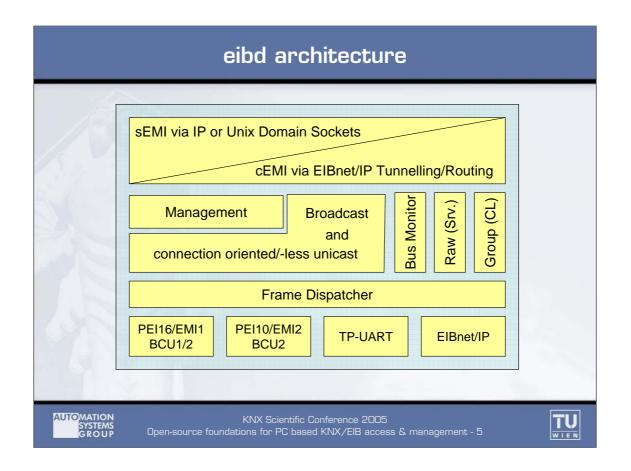
The architecture of eibd allows multiple clients to connect simultaneously. Higher-level tasks within eibd register with the frame dispatcher and state which frames (based upon addressing mode and destination address) they are prepared to process. To be able to serve multiple clients simultaneously, backends should deliver as many incoming frames as possible and leave filtering to the frame dispatcher.
