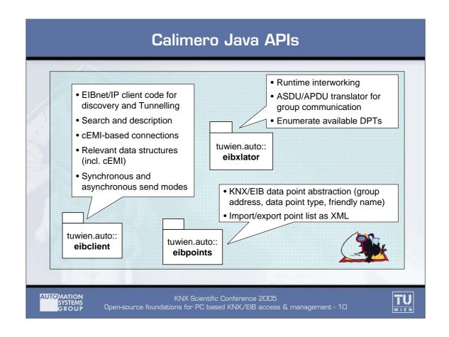
Calimero is a collection of Java APIs that together form a foundation for further EIB/KNX high level applications (including remote access and control). Still, these APIs can be used largely independently.
