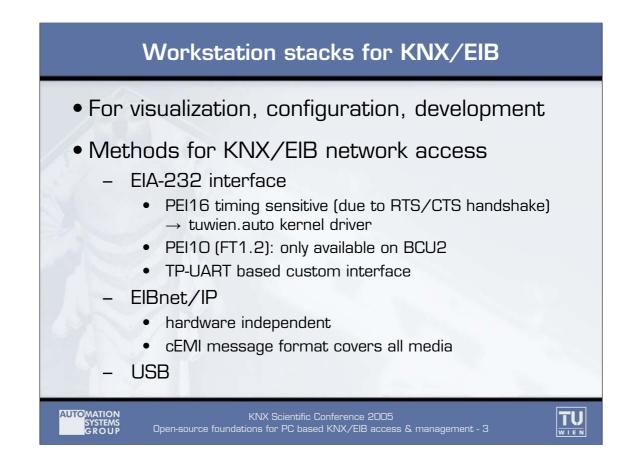
By its very purpose, most of the devices connected to a fieldbus are embedded nodes. Yet, there are applications whose resource requirements make it necessary to connect a general-purpose workstation (mostly a PC) to a network like KNX/EIB. This especially concerns visualization, configuration, and development tasks.
