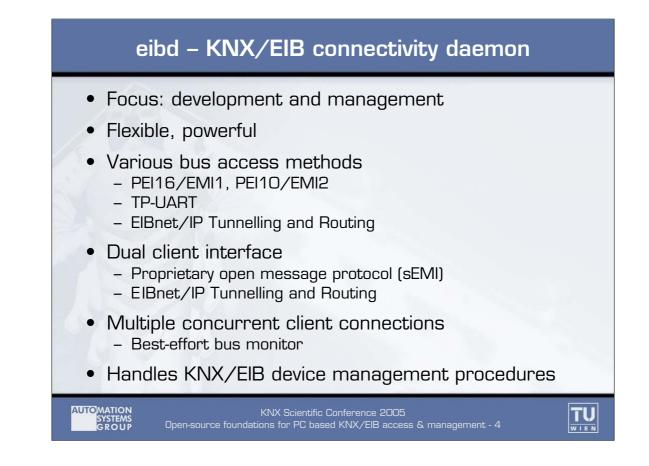
Within the BCU SDK project (which is covered in "Rapid Application Development for KNX/EIB BCUs"), a Unix daemon called eibd was created to cover access to the EIB/KNX TP1 network for development and management purposes.
