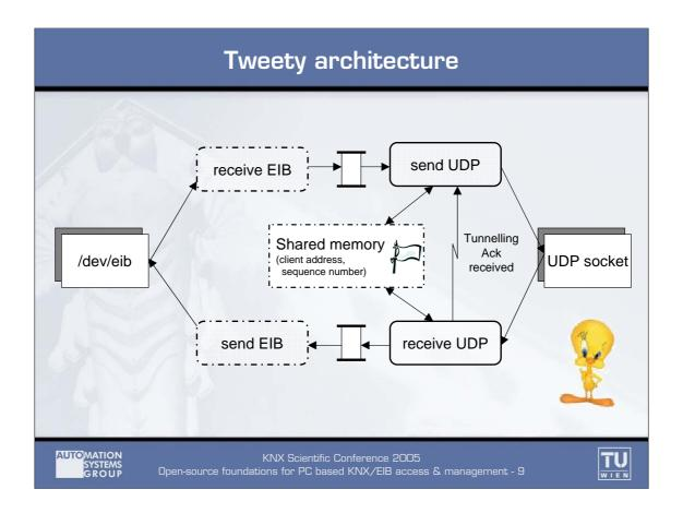
*Receive EIB:* This thread listens to the device node (e.g., /dev/eib) , and blocks until a new frame arrives. On reception the frame is passed to the pipe, and the thread returns to the blocking state.
