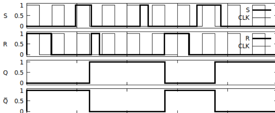
Figure 5.10: Simulation results of triggered RS flip-flop – model B
