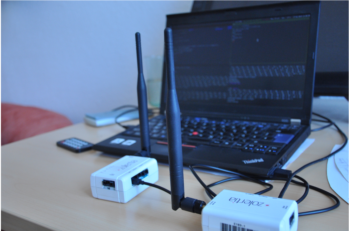
Figure 3.1: The test setup. The two devices are connected and powered via common micro USB cables.
