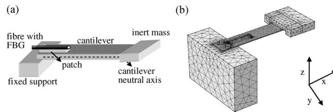
Figure 3.5: The image above, taken from [17], shows the operation principle of an optical FBG accelerometer
