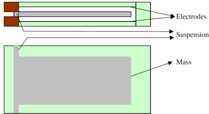
Figure 3.4: The image above, taken from [15], shows the operation principle of a capacitive accelerometer
