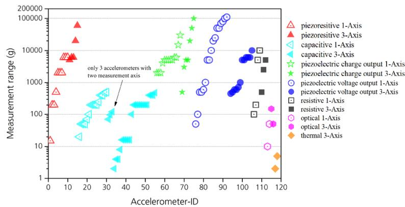
Figure 3.1: The image above, taken from [8], shows the upper measurement range of different accelerometers
