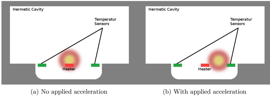
Figure 3.6: The images above, created from [18], shows the operation principle of a thermal accelerometer with and without applied acceleration
