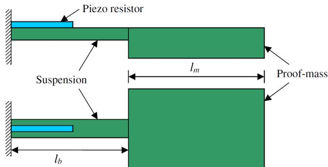
Figure 3.3: The image above, taken from [15], shows the operation principle of a piezoresistive accelerometer
