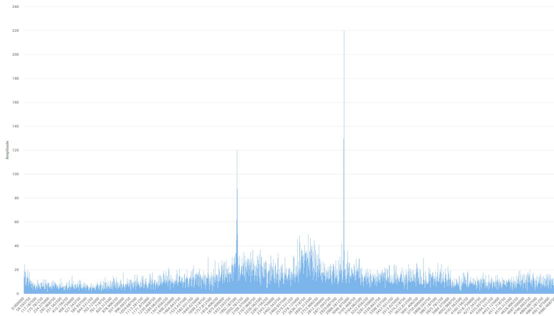
Figure 6.4: The image above shows the frequency spectrum while playing a sine at 3 kHz.
