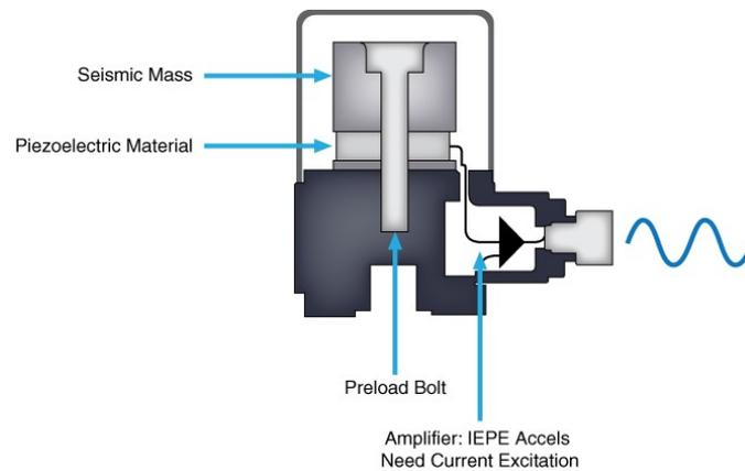
Figure 3.2: The image above, taken from [14], shows the operation principle of a IEPE accelerometer
