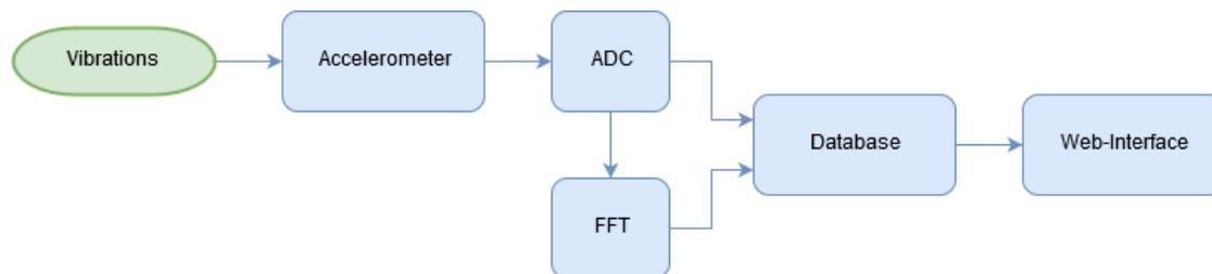
Figure 5.1: The image above shows the data processing chain.
