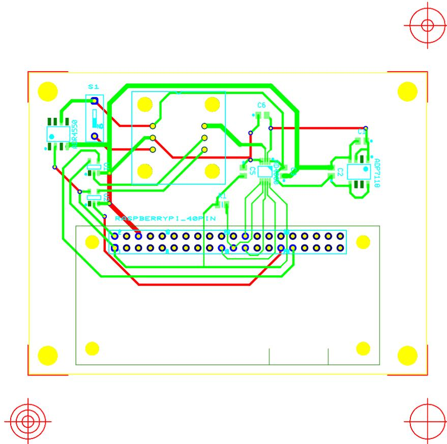
Figure 5.2: The image above shows PCB design of the circuit.
