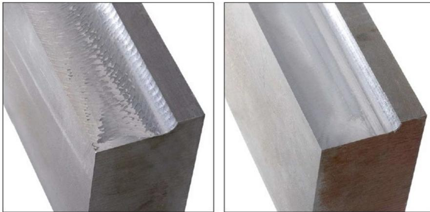
Figure 2.1: The image above, taken from [6], shows a workpiece with chatter on the left and one without on the right.
