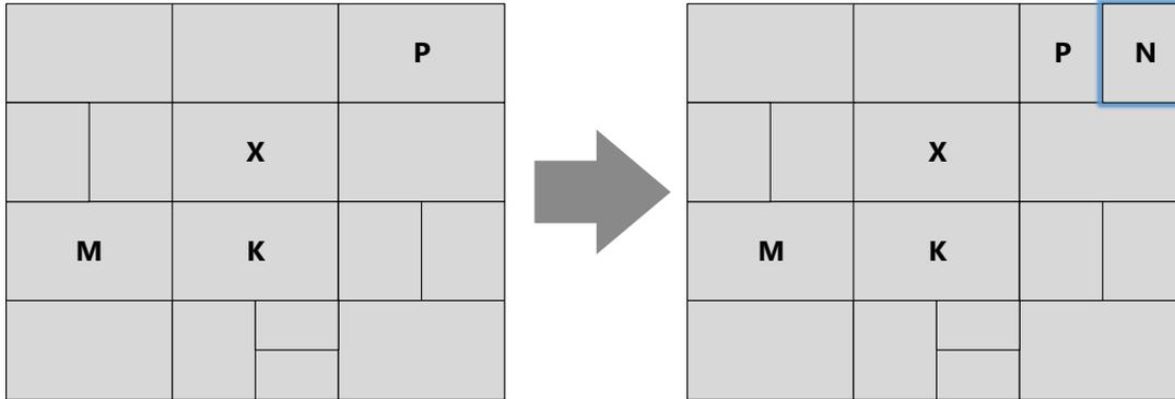
Figure 3.5: A 2D CAN network showing a split of zone P to accommodate a newly joined node N.
