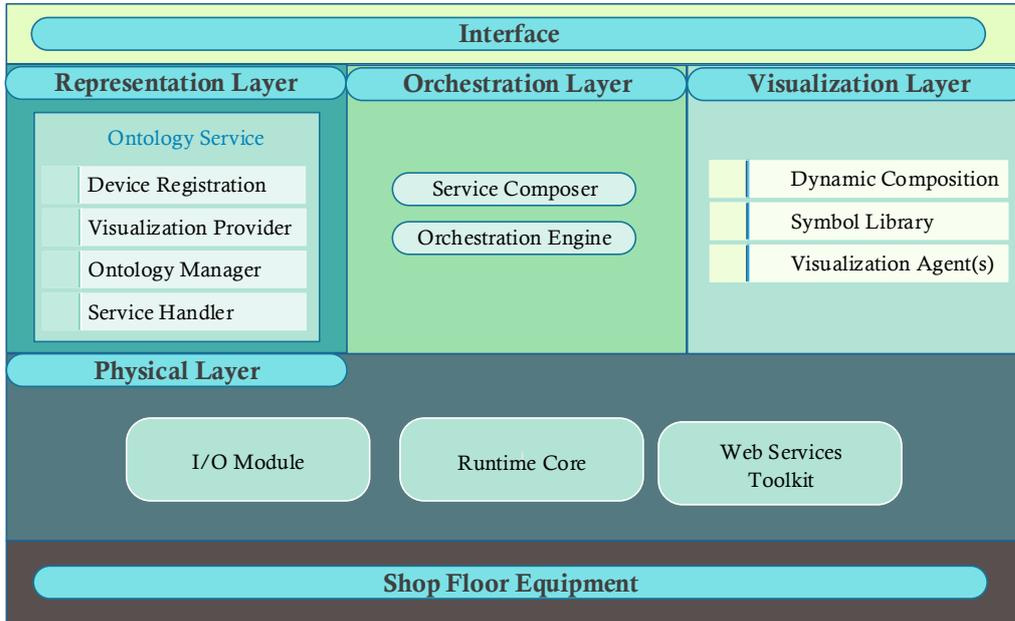
Figure 2.4: The eScop system architecture [45].
