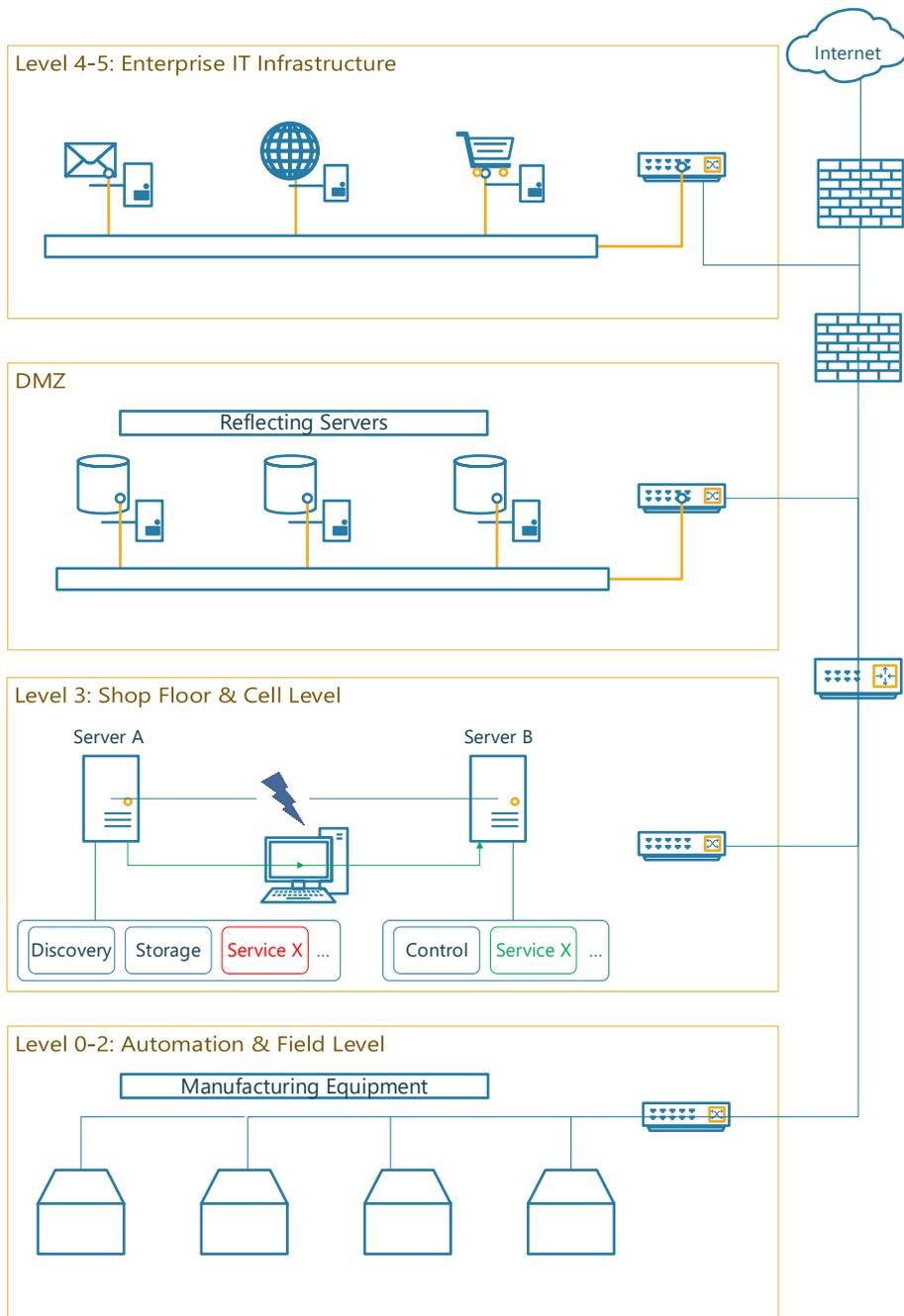
Figure 1.3: The envisioned resilient and robust SO manufacturing infrastructure. Service X on server A fails and is replicated on a different server (server B). With the link to the new service down, requests are re-routed through existing infrastructure to establish a new path for the continuity of data exchange.
