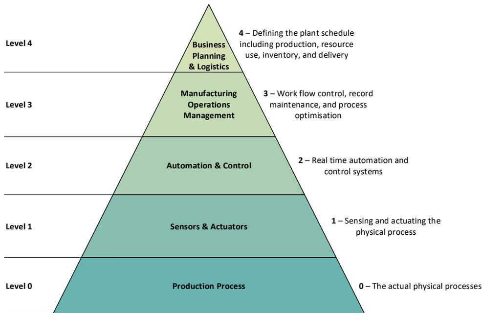
Figure 1.2: The five layers of the automation pyramid [23].
