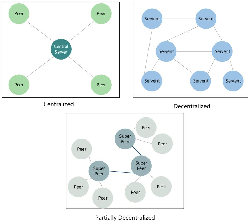
Figure 3.1: Representative examples of centralised (top left), decentralised (top right), and hybrid partially decentralised (bottom) networks.
