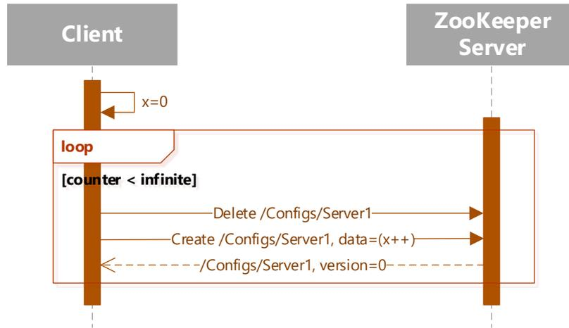
Figure 4.4: An example of a failure in conditional execution. The znode data is updated infinitely, but the version number remains the same.
