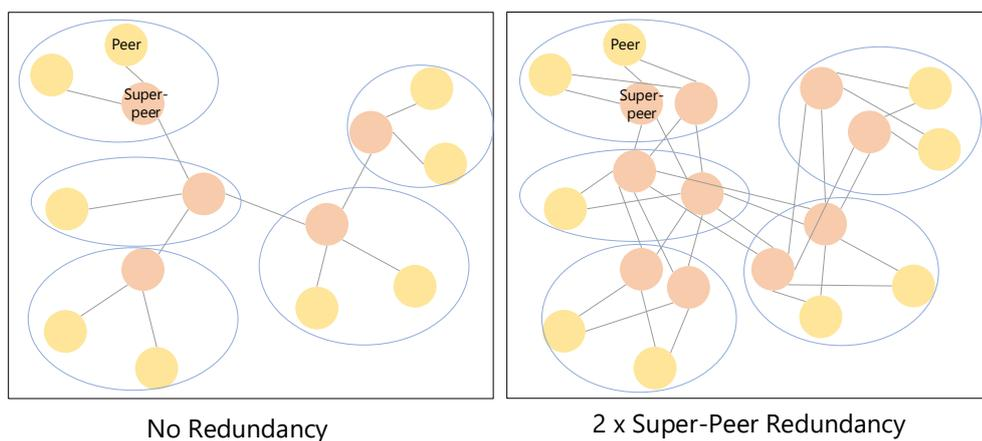
Figure 3.12: An example of a super-peer network with no redundancy and 2 super-peers redundancy as adapted from [173].
