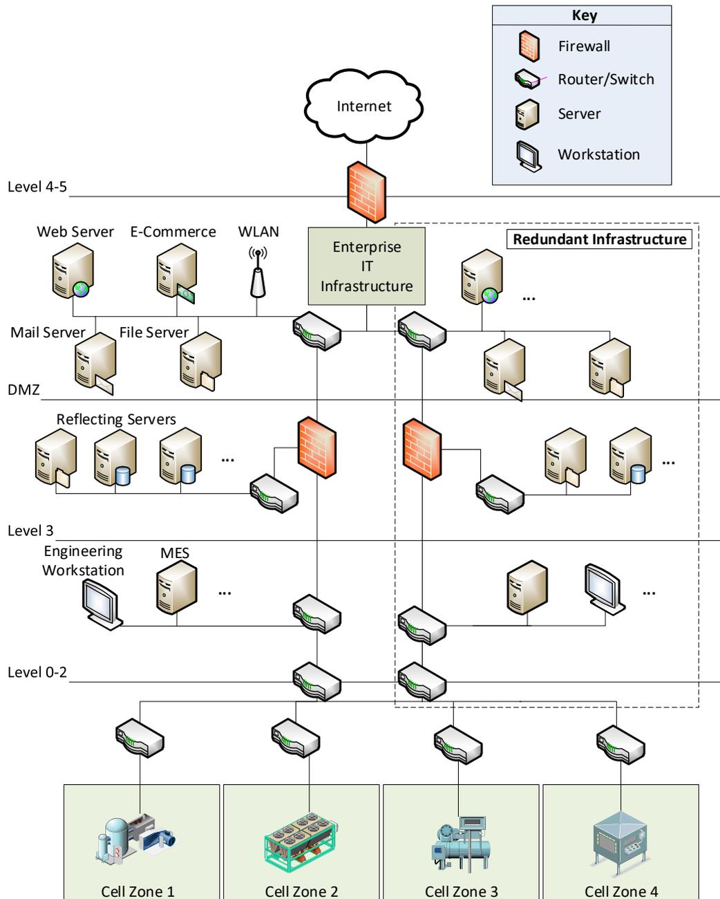
Figure 1.1: A typical manufacturing enterprise network architecture.
