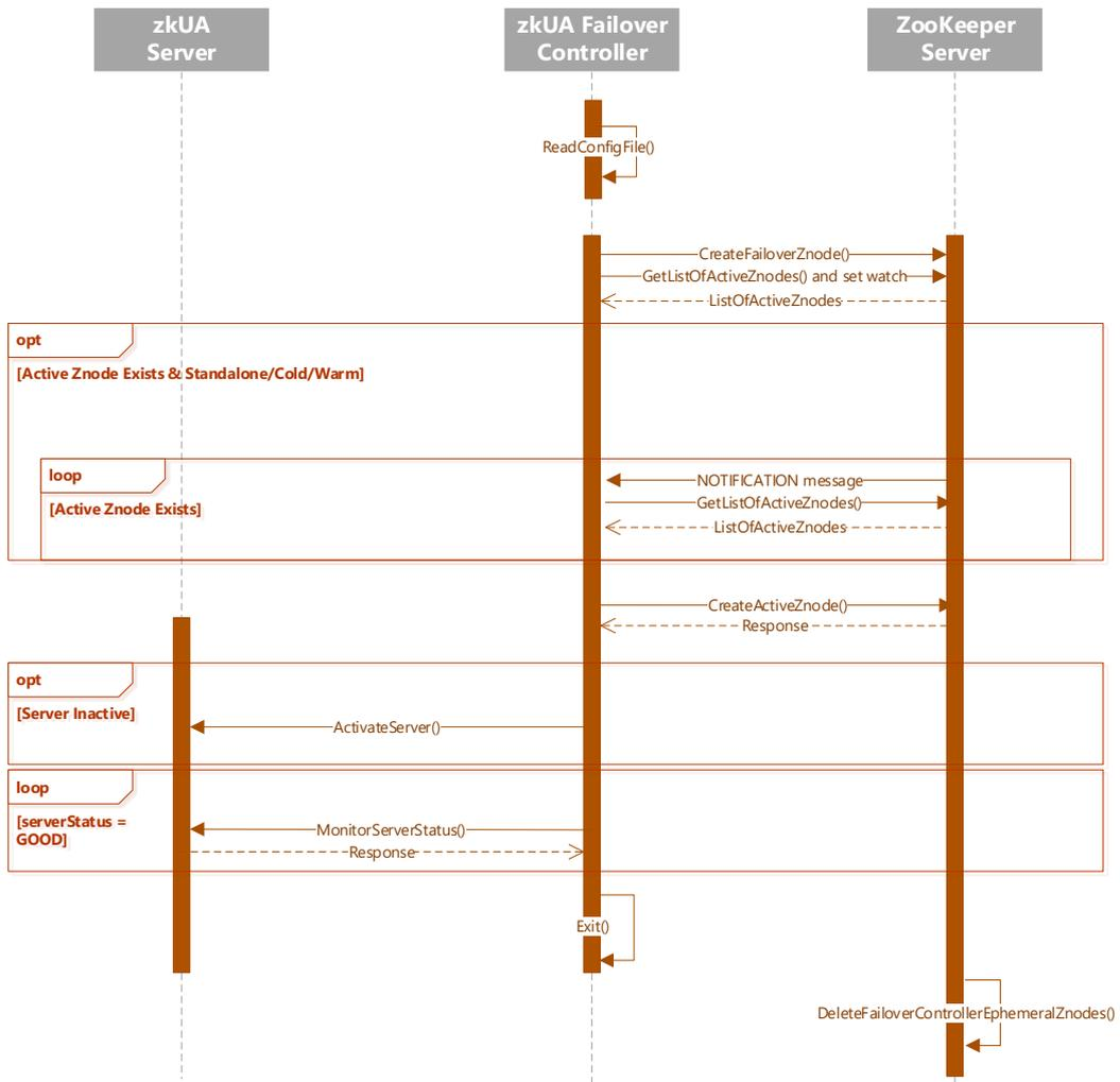
Figure 4.13: A UML sequence diagram showing the interactions taking place between a zkUA Server, a zkUA FC, and ZooKeeper.
