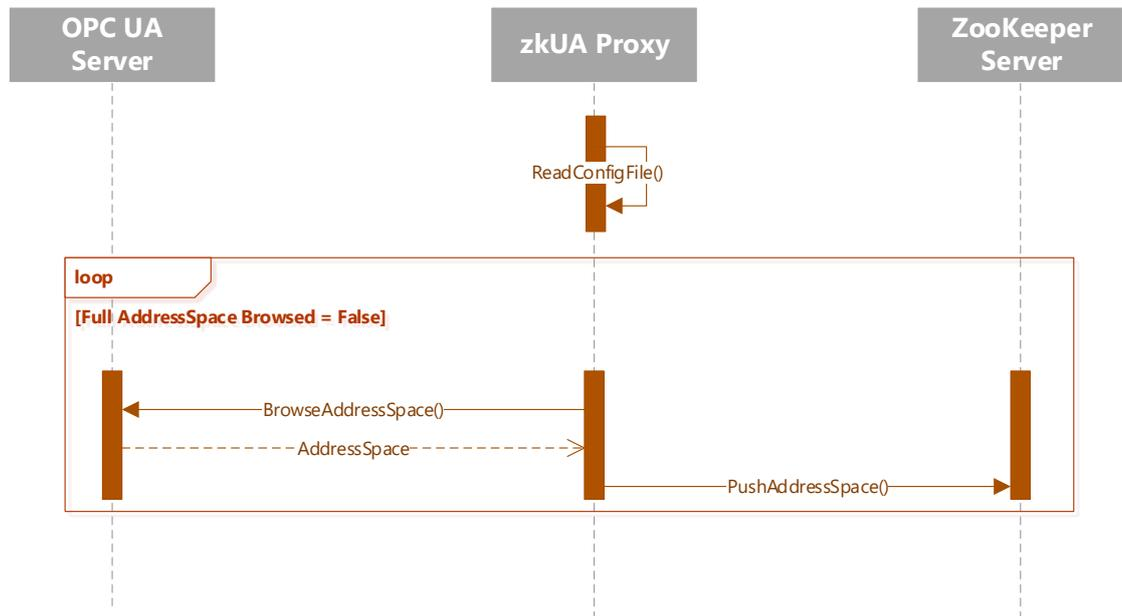
Figure 4.11: A UML sequence diagram showing the actions of a zkUA Proxy component.
