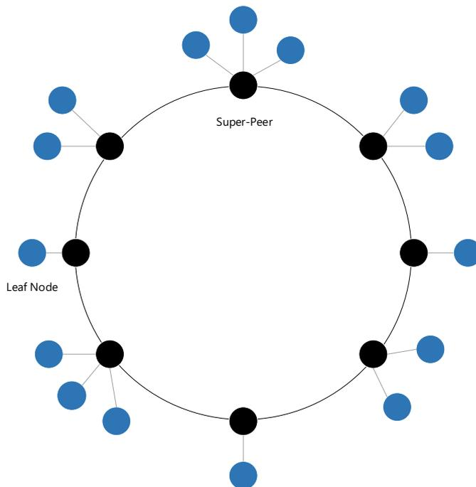
Figure 3.13: An example of a two-layer network in [174] with a Chord network upper layer and star-shaped connections with lower layer leaf nodes.
