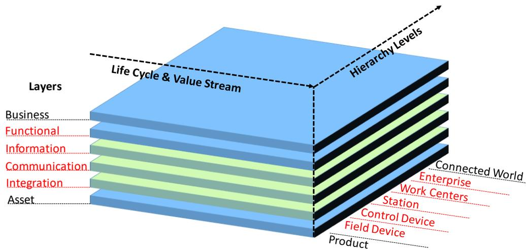
Figure 5.2: Translating the contributions to the RAMI 4.0. Addressed layers and hierarchical levels are highlighted in red.
