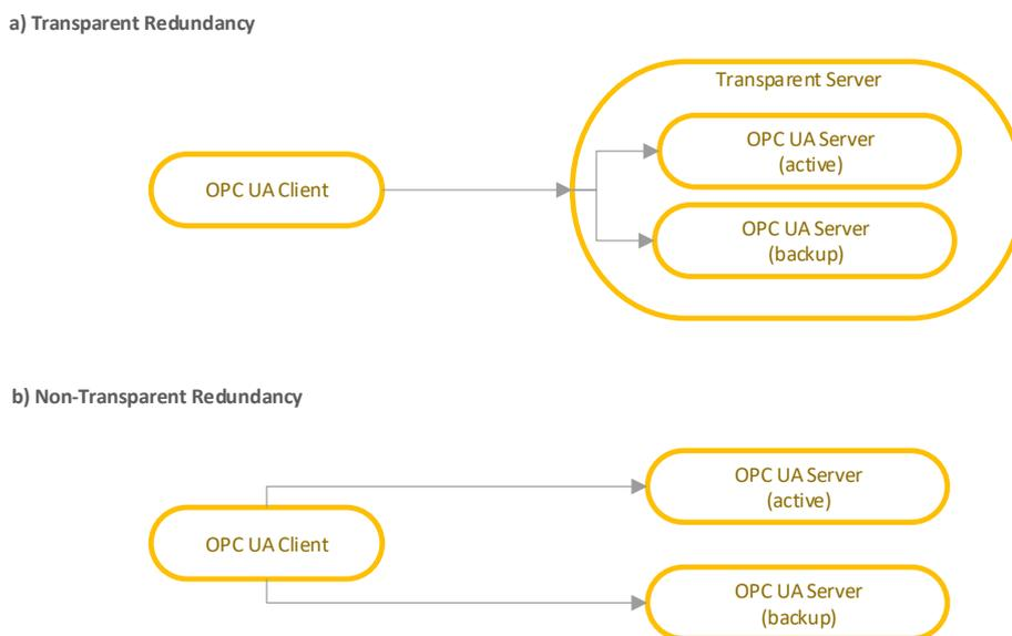
Figure 4.7: a) Transparent and b) non-transparent redundancy in OPC UA [133].
