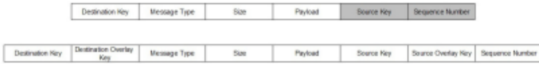
Fig. 3. The structure of a UDP Packet in the original Chimera implementation (above), and post-modifications (below).
