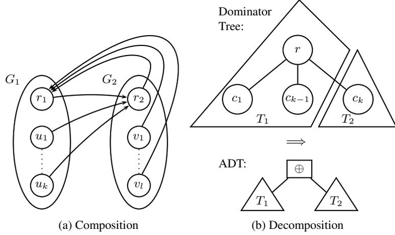
**Fig. 2.** Composition and Decomposition of Reducible Flowgraphs.
