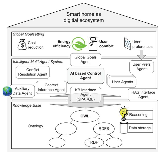
Fig. 1. Schematic Overview of the ThinkHome System Components
